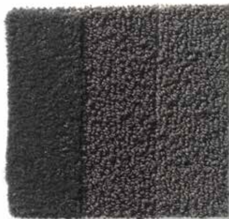
902-497A Mid Dull Deep Acid Heatset Cut 902-497A Mid Dull Deep Acid Heatset Loop 902-497A Mid Dull Deep Acid Non-Heatset Loop
